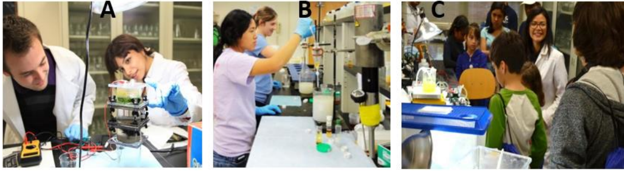
Fig.3. Civil and environmental engineering students working on various research-education based projects (A. Graduate and undergraduate students working on a microbial desalination cell which treats the wastewater and salt water simultaneously while producing electricity; B. High school students learning the biodiesel purification process; C. A graduate student provides educational outreach to the Starkville community in the Water-Energy laboratory of the Civil and Environmental Engineering department)
