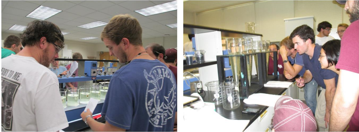
Fig.1. Civil and Environmental engineering students performing water treatment experiment (coagulation-flocculation-sedimentation-filtration techniques)
