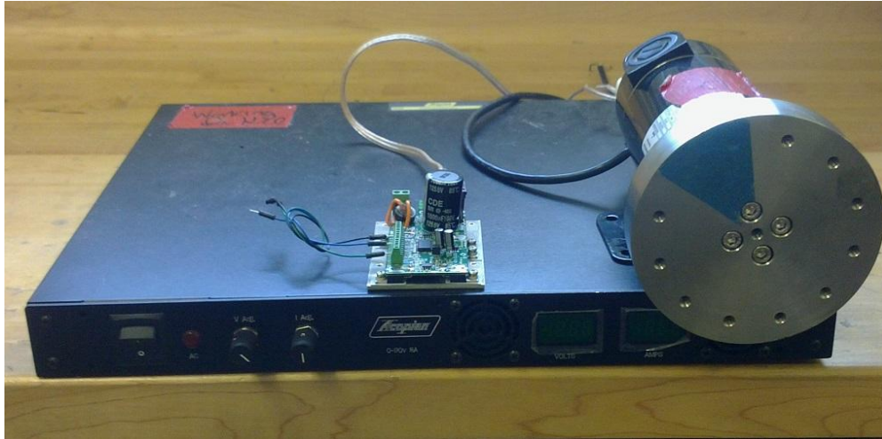
Figure 2: DC motor and flywheel plant with power supply and H-bridge to help students explore various controller designs.
