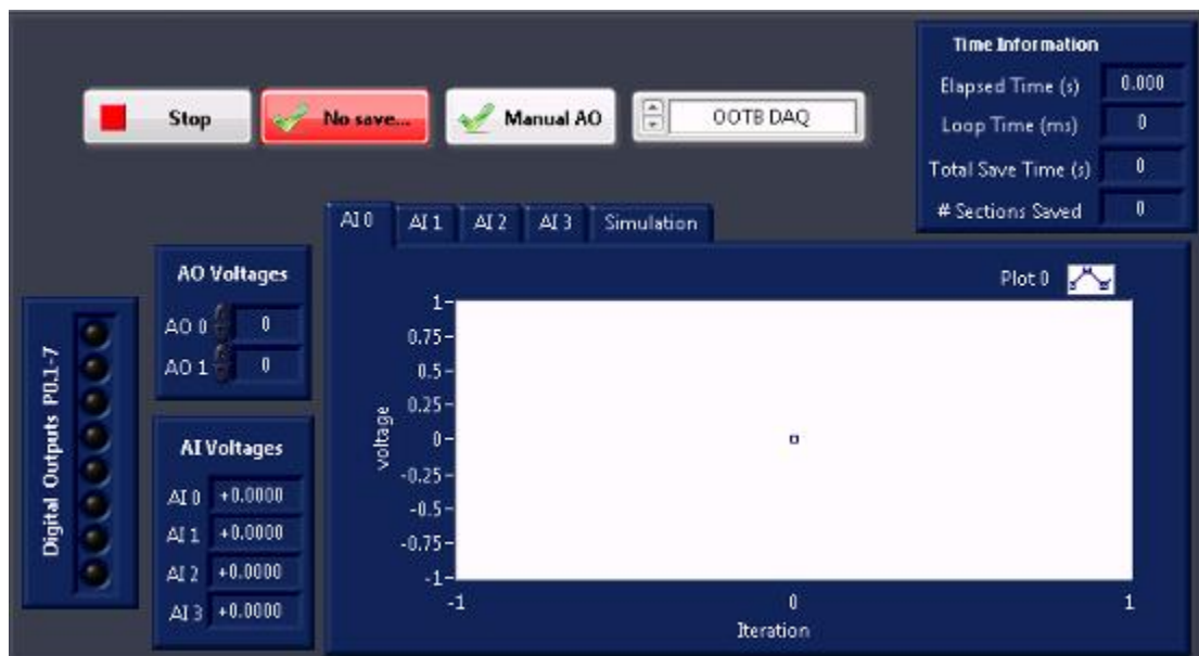
Figure 7: Front Panel view of student framework code in LabVIEW. Students use this code as a foundation to complete all lab experiments, which has built in functionality for analog in/out, digital in/out, file saving, and data graphs.
