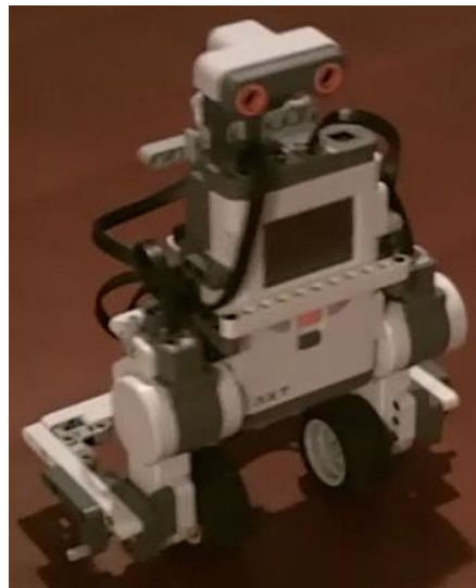
Figure 4: Self-balancing Lego NXT Segway with gyroscope for tilt sensing.
