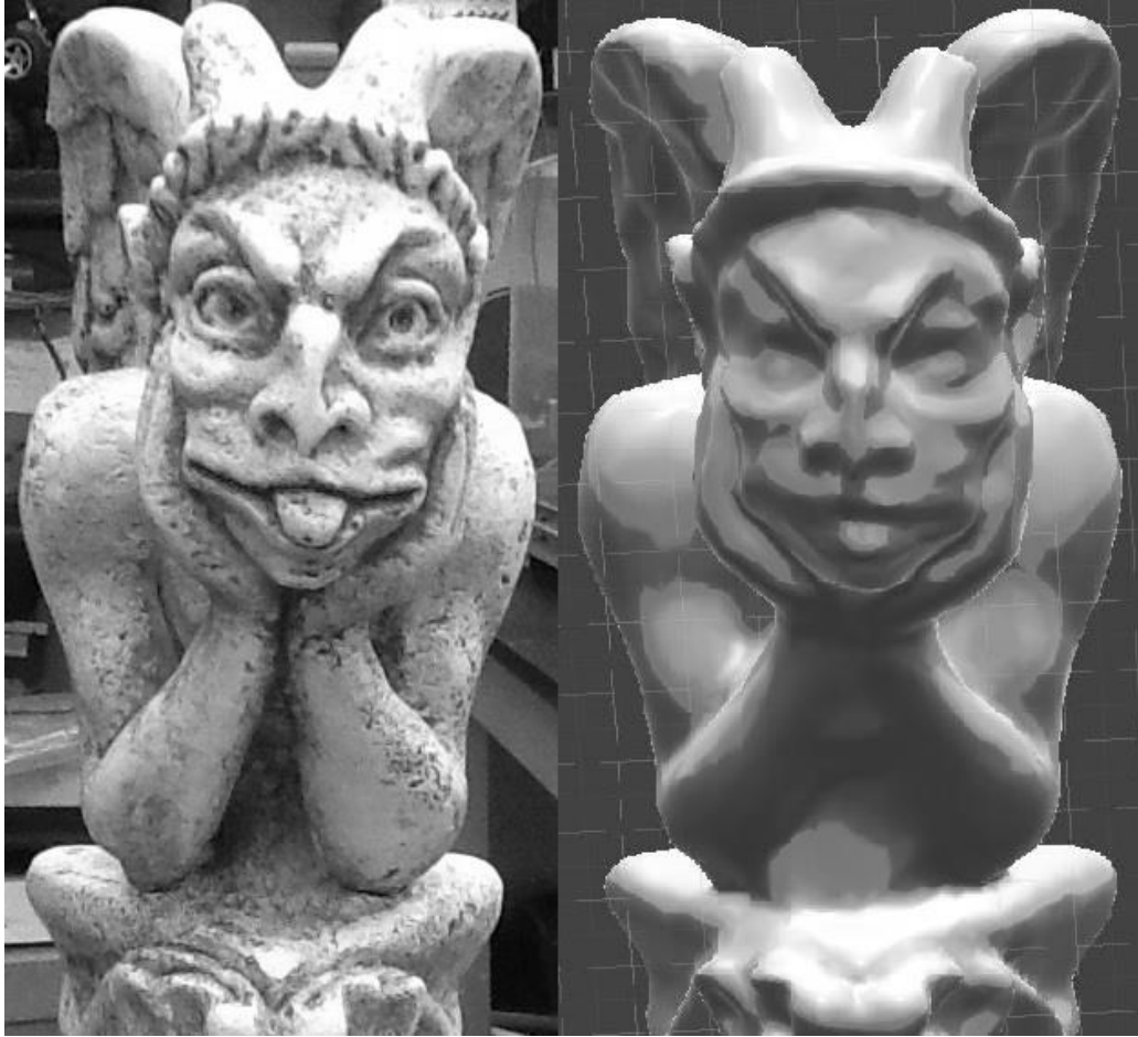
Figure 6: An example of an object that was turned into a 3D point cloud by using 123D Catch. The object on the left is the object of interest, a gargoyle and the object on the right is the 3D model created by 123D Catch. The build-in camera of an iPad was used to collect the photos for use in 123D Catch.
