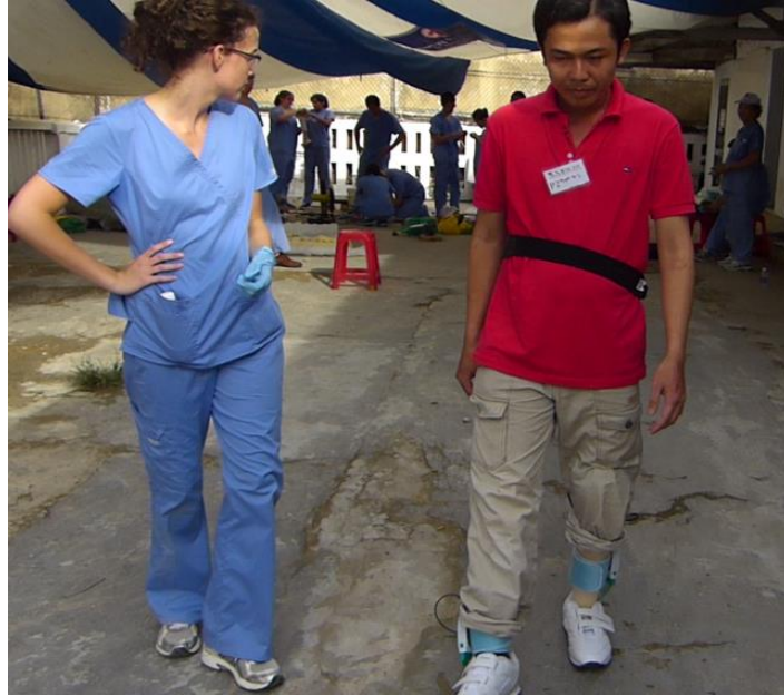
Figure 8: Patient walking with F-Scan system: sensors in the shoes and wireless transmitter around the waist.
