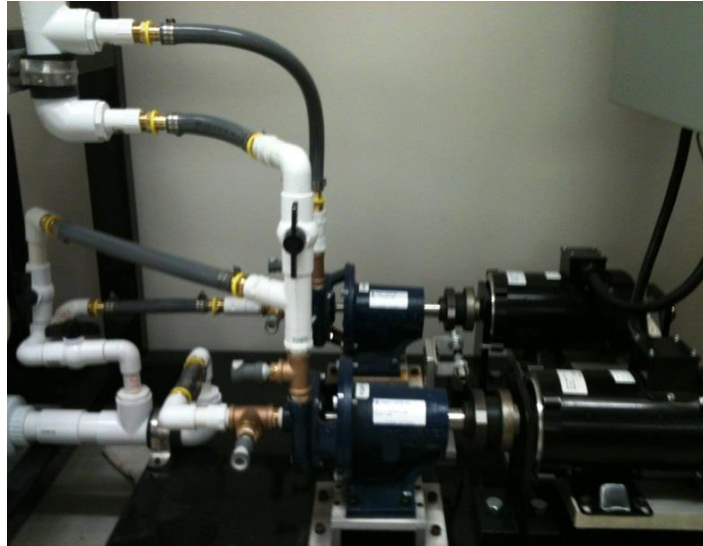
Figure 4: Current design of flex-hose/PVC pipe network
