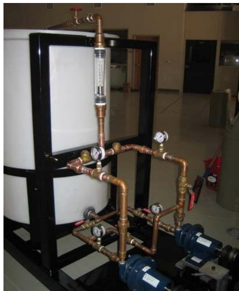
Figure 3: Front view of the pipe network of the centrifugal pump test bed as of 2006
