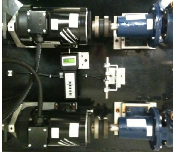
Figure 2: Top View of Motor-Pump Assembly, Force Probe, and Optical Sensors
