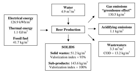
Figure 2. Mass balance applied to Unicer SA breweries representing specific values, i.e., values per m<sup>3</sup> of produced beer [13].
