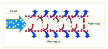
Figure 3. Schematic showing the principles of crossflow filtration [32].
