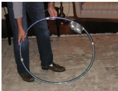
Figure 7. The unbalanced hula-hoop will hop if rolled fast enough.
