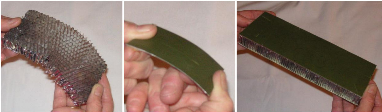
Figure 2. A simple sandwich structure illustrates the power of the parallel axis theorem in design for flexure
