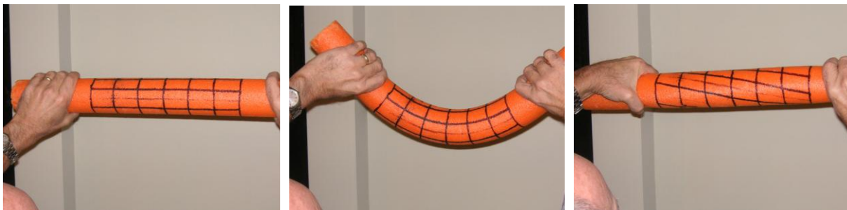
Figure 1. A water noodle is used to demonstrate flexural and torsional deformation.
