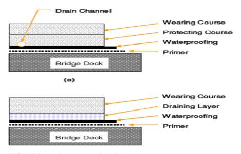
FIGURE 3: Drainage systems in Bridge deck pavements: (a) Traditional system; (b) Proposed new system.
