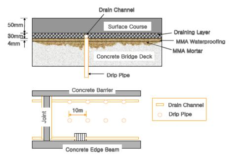
FIGURE 4: Section and plan view of bridge deck pavement with drainage system
