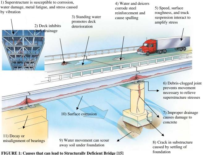
FIGURE 1: Causes that can lead to Structurally Delicient Bridge [15]
