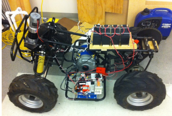
Figure 5 A Remote Control Driving and Steering System on an ATV Chassis
