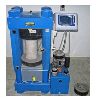
Figure 5: Compressive strength test of concrete.
