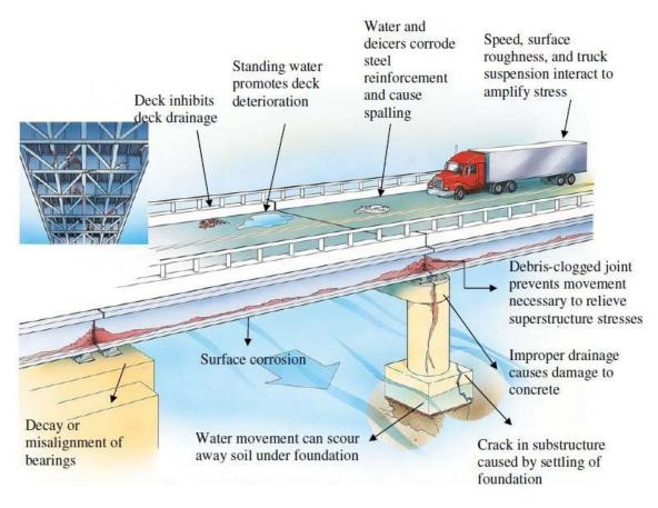
Figure 1: Corrosion Causes
