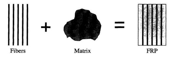
Figure 2: Fiber-Reinforced Polymer Breakdown
