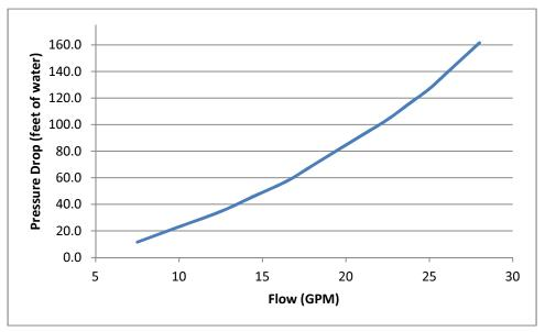
Figure 7: CPC Fitting Pressure Drop vs. Flow Rate [4]
