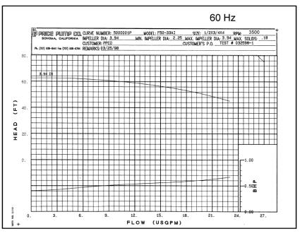
Figure 2: Manufacturer's Pump Curve [1]
