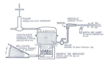
Figure 1: Shipboard Byzantine Flamethrower
