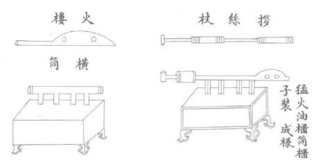
Figure 6 Components of the Chinese Flamethrower (Fierce Fire Oil Projector)
