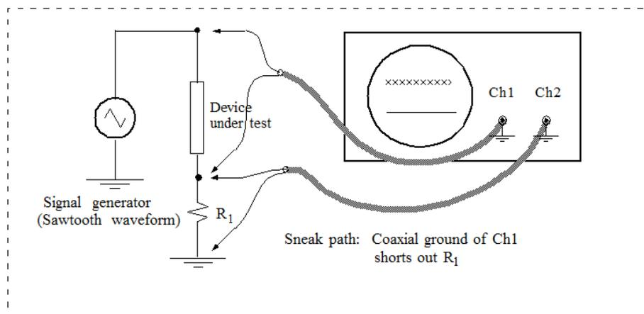
Figure 1(a) Sweep measurement sneak paths
