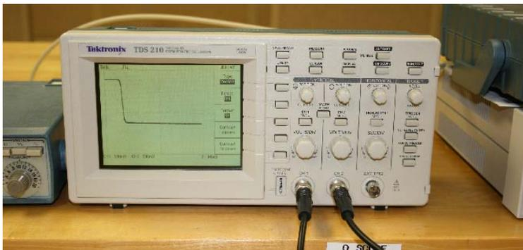
**Figure 4(b).** Photo snapshot of XY output trace courtesy of the test frame of Figure 4(a). Because the current sensing topology inverts the signal, the y-axis corresponding to collector current represented by Figure 4(c) is negative
