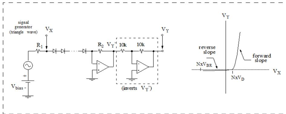
Figure 3(a) Diode test circuit
