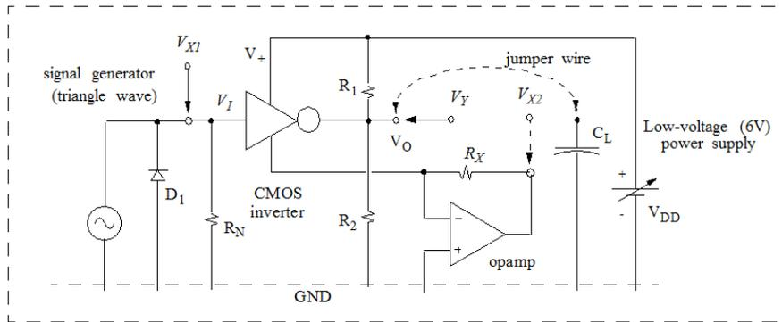
**Figure 5(a)** Test set-up for (1) evaluation of CMOS transfer curve  $V_O$  vs  $V_I$  and (2) inverter transition current [4]. For transfer characteristics  $V_O$  vs  $V_I$ , node  $V_I$  is wired to CH-1 and  $V_O$  is wired to CH2- of the oscilloscope (labeled as  $V_{X1}$  and  $V_Y$ , respectively, in the figure) and the Oscilloscope is set to the X-Y mode.
