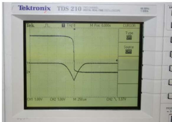
**Figure 5(b).** Photo snapshot of inverter characteristics. The upper trace = CH-2, represents the CMOS transfer curve trace. The lower trace is CH-1 and represents the transition current profile, inverted by the opamp topology. The traces are stabilized by setting the trigger mode to the CH2 falling edge.
