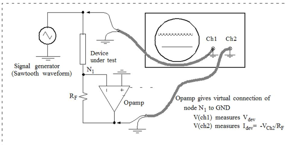
**Figure 2.** Device I-V measurements using a virtual ground. The inputs of the opamp are not connected, but are virtually the same courtesy of the high voltage gain of the opamp for which  $(V_+ - V_-) = V_o/A_V$ , where  $A_V$  is usually on the order of  $10^4$  V/V or higher.
