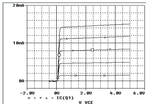
**Figure 4(c).** pSPICE [3] simulation-generated BJT characteristics for comparison to Figure 4(b). Measurements of each Oscopce trace are made for determination of [2] (a) forward current gain  $\beta_F$  and (b) forward Early voltage  $V_{AF}$  (slope parameter for the saturation regime)
