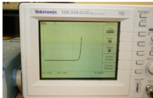
Figure 3(c) . XY output trace for the 3(a) test circuit
