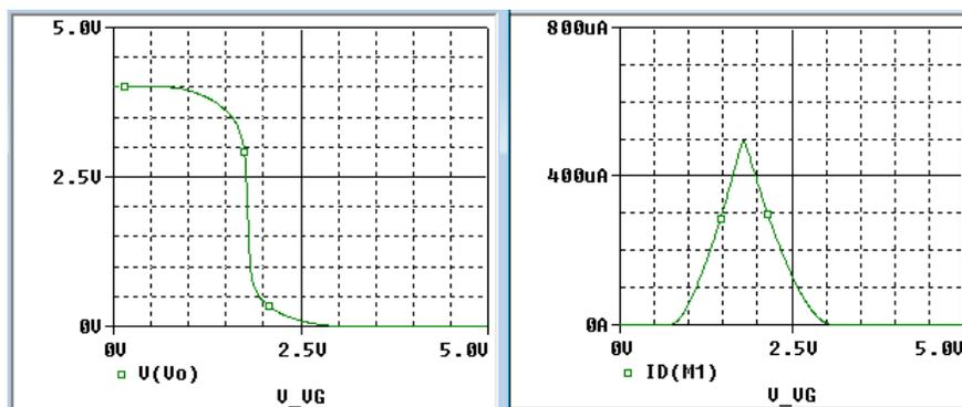
**Figure 5(c).** pSPICE [3] simulation comparisons to the traces of Figure 5(b)
