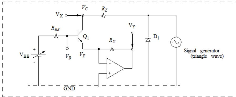
**Figure 4(a)** Test frame for measurement of *npn* BJT characteristics. Oscilloscope CH-1 is wired to node  $V_X$  and Oscilloscope CH-2 is wired to node  $V_Y$ .
