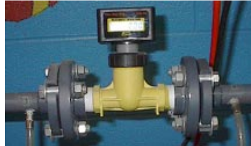
FIGURE 2. A SCHEMATIC OF A TURBINE-TYPE FLOW METER.
