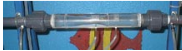
FIGURE 4. A SCHEMATIC OF THE VENTURI METER.
