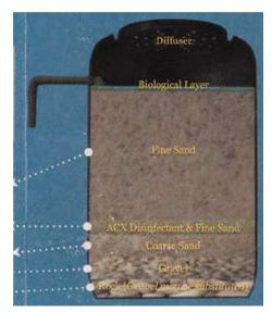
Figure 4. Modified BSF Schematic Source: AquaClara International
