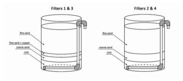
Figure 5. mBSF (on left) and CBSF (on right)
