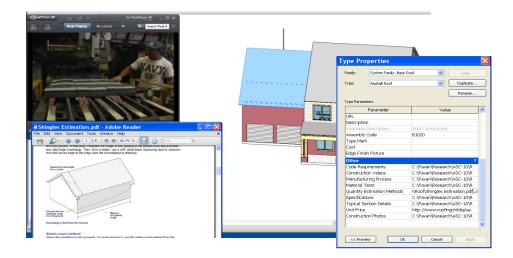
Figure 4: Retrieved manufacturing video and estimation guidelines for Asphalt Shingles roof component
