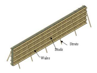
Figure 3: Knowledge repository 3D model of wall formwork system
