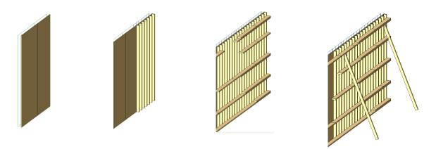
Figure 5: Erection sequence of wall formwork system
