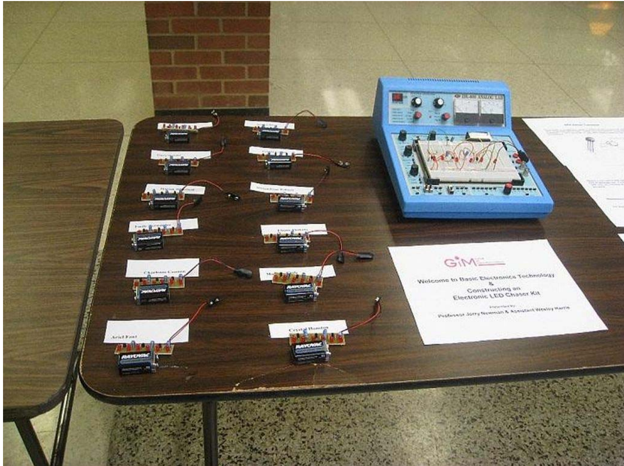
Figure 6. Finished LED Kits and a Trainer-Wired Kit
