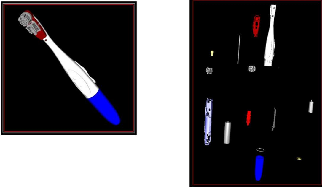
Figure 1: Model of a Mechanical Power Toothbrush
