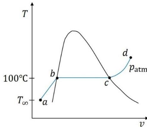
Fig. 1:  $T$ - $v$  diagram for the vaporization of water at constant pressure (see Moran et. al<sup>4</sup>).
