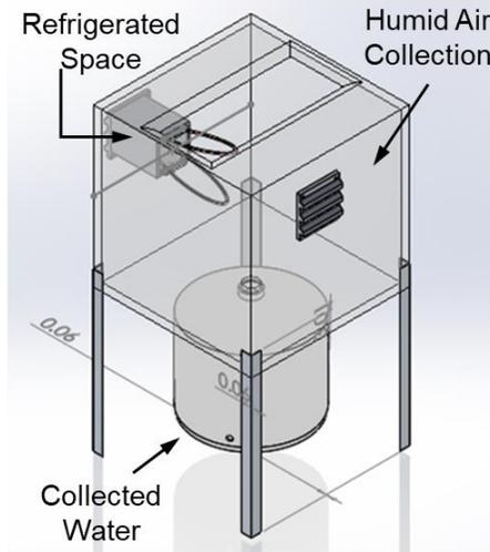
Fig. 4: Solar powered water collection via dehumidification.
