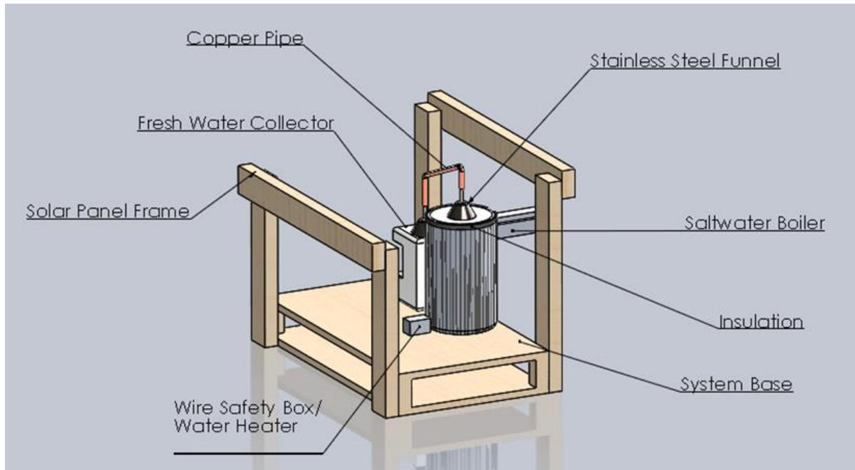
Fig. 2: Basic solar powered desalination plant.
