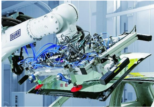
Figure 4. Complex End of Arm Tooling Used to Place a Windshield on a Car
